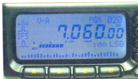
Detail of the liquid crystal display, showing the band scope along its bottom edge.
