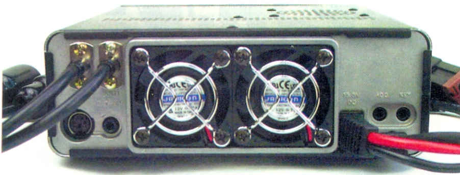
The Power Amplifier is cooled by two fans mounted on the rear panel.
