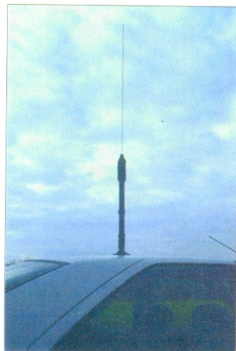
ATAS-100 mobile antenna, which is made to match the FT-847 and FT-100.
